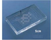
Shown is a microfluidic chip from the Fluidigm web site. This rubber like material is filled with 20 micron sized sample and control paths that are connected to pressure solenoids and fluid sources.
